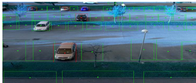
Fig. 11. Result of the pre-trained Mask R- CNN model detected an empty space with a green rectangular box and a red rectangular box for a vehicle
